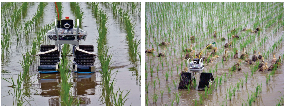
Figure 19 Small weeding robot for paddy fields, nicknamed “Aigamo Robot”
