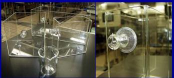
(Use all glassware tank, and stainless steel mesh net to Drainage for waste water avoid the contamination of unknown chemicals from equipments.)
