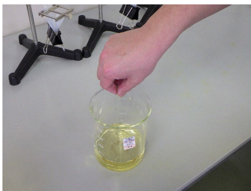
Photo 5-14. Stirring of a sample with a glass rod
