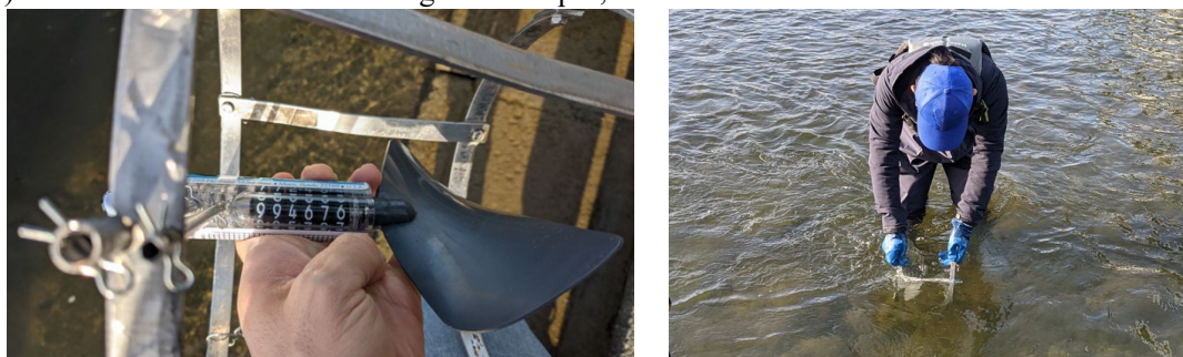
Photo 3-11. Measurement of flow velocity with flow meter
