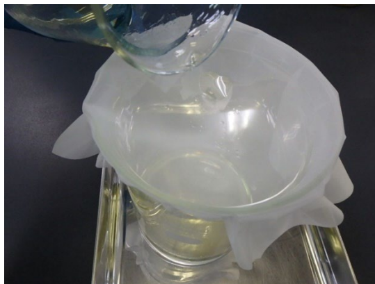
Photo 5-20. Filtration of water to collect samples
