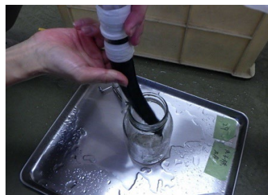
Photo 3-14. Transfer of samples from a bottom pipe (or cod end) to a container
