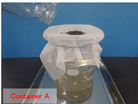
Photo 5-1. Filtration of impurities through a net
