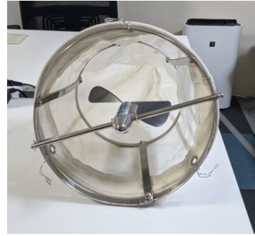
Photo 3-6 Case 2. An example of fixation of the flow meter with a metal frame
