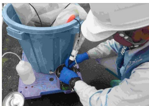
Transfer of samples from a bottom pipe (or cod end) to a storage container
