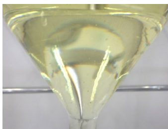
Upper and middle part At the start of density separation
