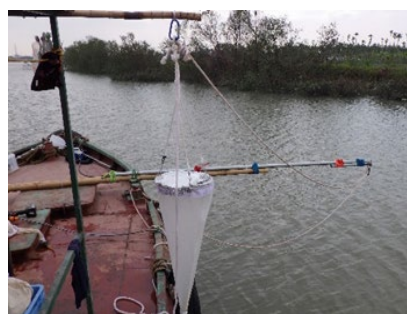
(Left: a frame to hang the net, Right: a pipe fixed to the existing frame)
