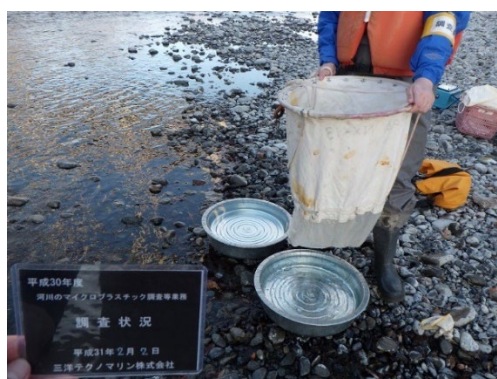
Filtration of river water with a net with 0.1 mm mesh openings
