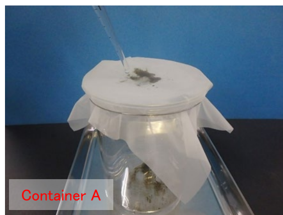
Photo 5-6. Drop of the samples sticking on the net into container A
