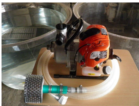
Photo 4-6. An example of a pump and a strainer
