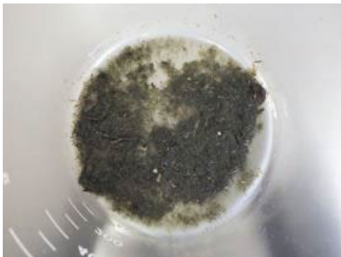
After drying for 2.5 hours (top view); the end of drying process
