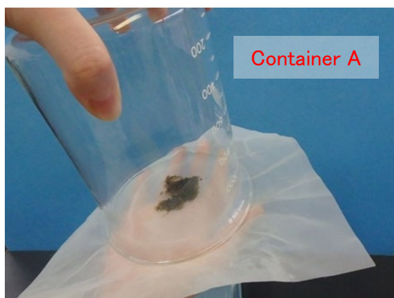
Photo 5-5. Putting container A on the net with samples side facing inward
