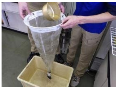
Photo 3-13. Collection of samples in a bottom pipe (or cod end)
