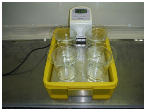
Photo 5-10. Warming of containers in a water bath
