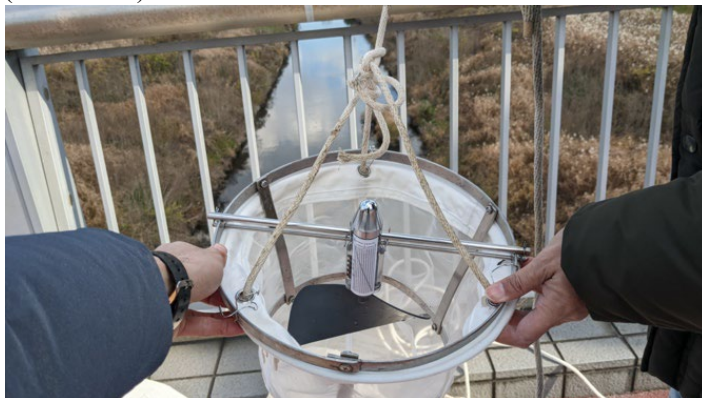
Photo 3-8. An example of fixation of plankton net
