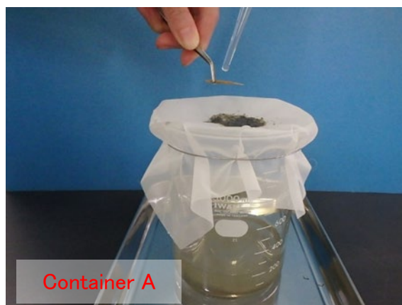
Photo 5-2. Removal of large impurities
