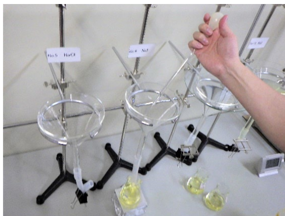
Photo 5-19. Rinsing out the remaining samples
