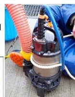
Pump Tsurumi Manufacturing 50TM2.45 Flow rate: 80 L/min
