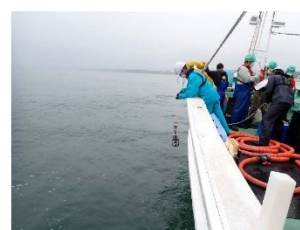
Measuring water temperature, salinity, etc. with a CTD
