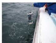
① Lowering the bottle 1: Used for rapid analysis of tritium
