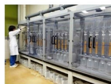
Separating and refining strontium with a cation exchange resin
