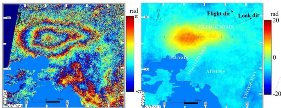
A Methodology to Validate the InSAR Derived Displacement Field of the September 7th, 1999 Athens Earthquake Using Terrestrial Surveying. Improvement of the Assessed Deformation Field by Interferometric Stacking (<https://www.mdpi.com/1424-8220/8/7/4119>)
