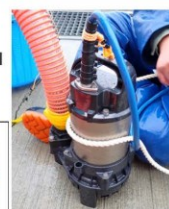
Pump Tsurumi Manufacturing 50TM2.45 Flow rate: 80 L/min
