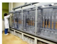
Separating and refining strontium with a cation exchange resin
