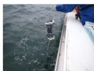
① Lowering the bottle 1: Used for rapid analysis of tritium
