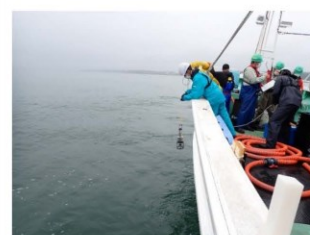
Measuring water temperature, salinity, etc. with a CTD
