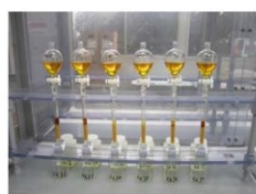
Separating and refining plutonium with an anion exchange resin
