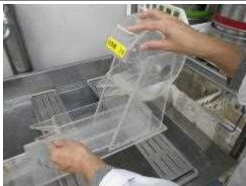
Use of Folsom splitter Splitter is moved back and forth to mix thoroughly, then the sample is divided.
