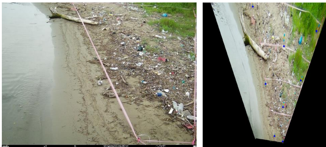
Figure 2.1.4. Image of the beach taken by a stationary camera (left) and image after projection transformation (right)
