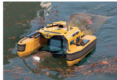
The JELLYFISHBOT marine drone collects substances floating on the water (seaweed, plastics, and toxic substances).
