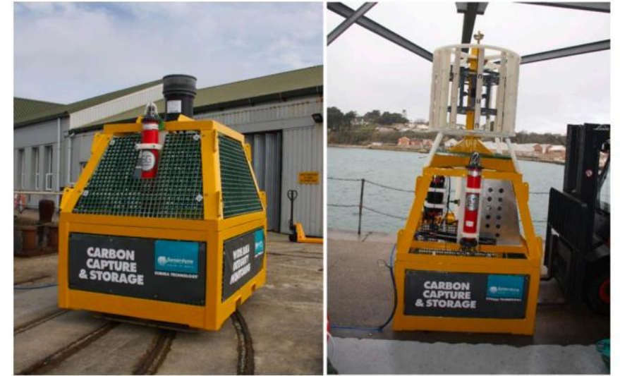
The active sonar lander prior to deployment on harbour trials
