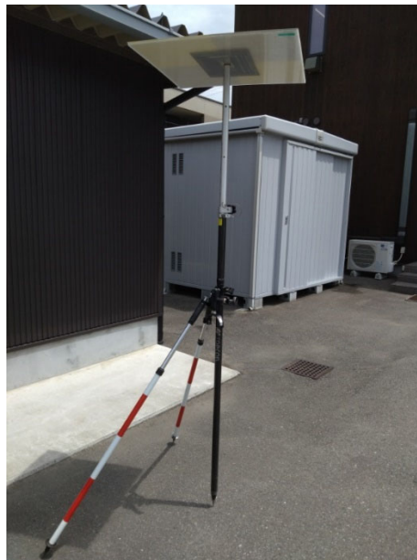
Figure 4. Example of installation of a stereo ground control point targets
