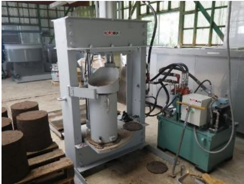
Press machine for manufacturing the fertilizer (Made by Kotobuki Sangyo Corporation)
