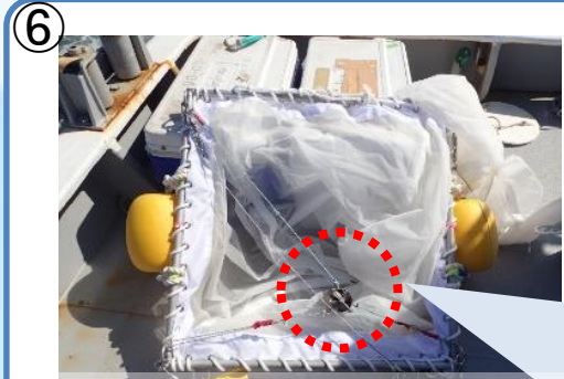
Neuston net with flow meter
