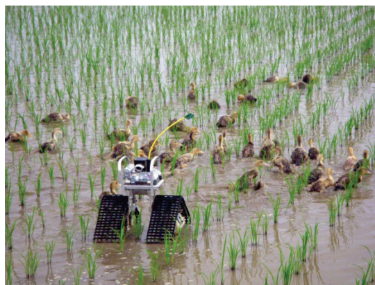
Figure 19 Small weeding robot for paddy fields, nicknamed “Aigamo Robot”
