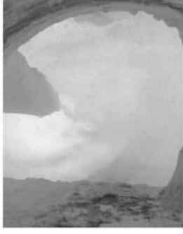
Inside of a kiln (Clinker temperature is around 1450°C)
