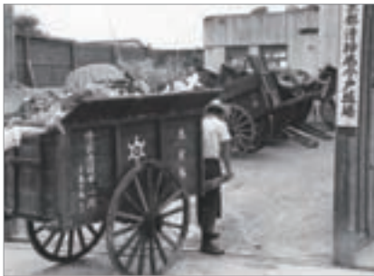
A cart used to collect waste from homes. Collected waste was reloaded onto special automobiles or vessels at waste collection sites or on the streets to be transported to incineration sites or landfills.
