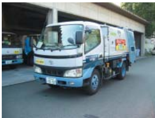
Mechanical waste collection vehicle (packer car) Source: HP of the Resource & Waste Recycling Bureau, Yokohama City
