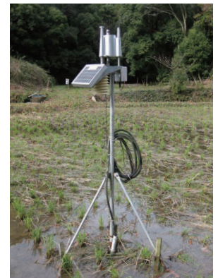
A sensor system for meteorological data
