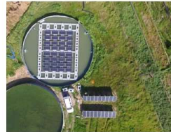
Floating Solar panels in WWTP Kraaifontein, South Africa Image: University of Cape Town (UCT)
