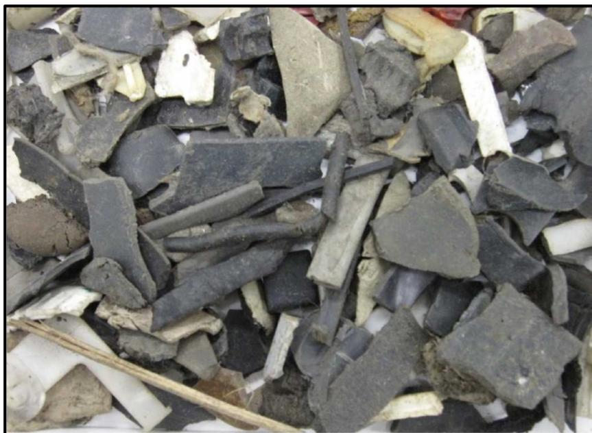
図3.1.3-28 破碎粒度小の受入A S R ( 2 )の状
