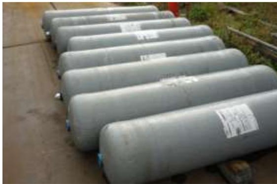
図2.4 CNGボンベ (CFRP + GFRP)
