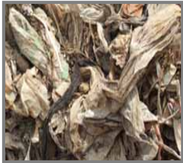
mined wastes from dumpsite
