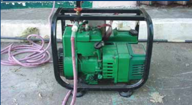
A hybrid 5 hp biogas run generator
