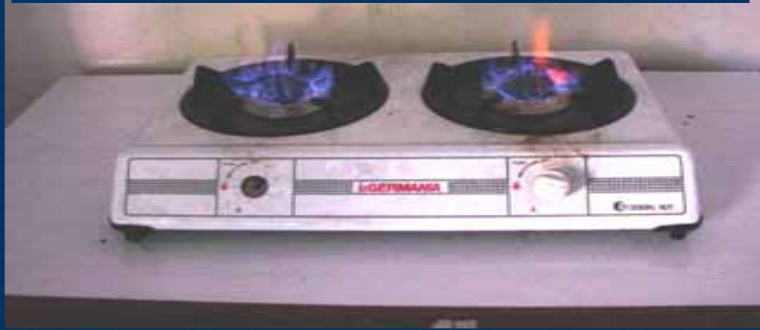
Cooking: An LPG modified double burner biogas stove
