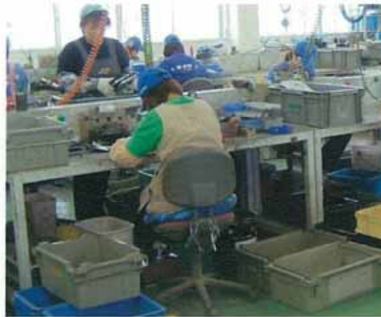
Dismantling and separation by hand
