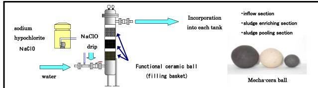
[Principle] Air agitation triggers a catalytic reaction after sodium hypochlorite is added and water (or mecha-cera water) that touches the ceramic in the system is injected into the treatment plant. Mecha-cera water with sufficient oxidizing capability resolves the organic substance in wastewater or sludge into CO<sub>2</sub> (carbon dioxide), H<sub>2</sub>O (water), and N<sub>2</sub> (nitrogen) and is effective for reducing the volume of the sludge.
