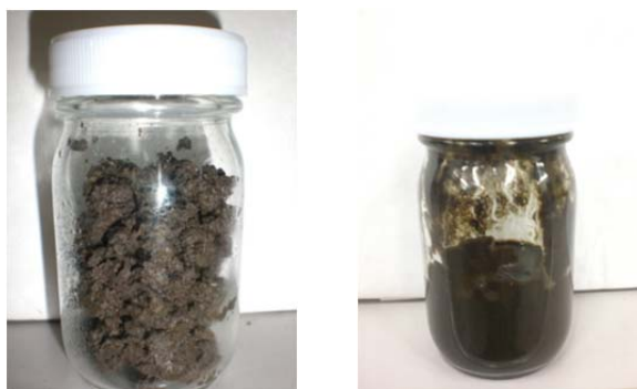
Fig.2-2 Appearance of initial feedstock and after hydrothermal treatment
