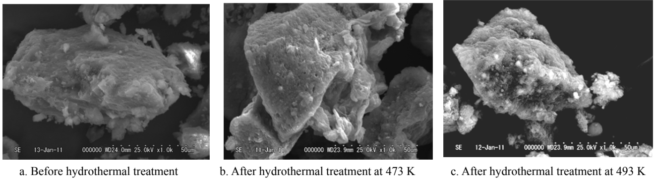
Fig.2-14 SEM photograph of sludge and solid residues
