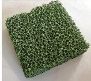
$\text{Cr}_2\text{O}_3$ -coated honeycomb
