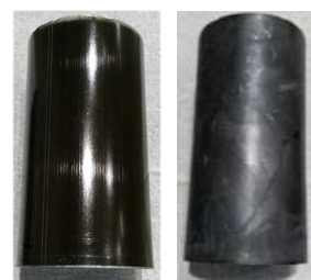
Photo 1 Monolithic specimens solidified with epoxy resin (left) and modified sulfur (right).
