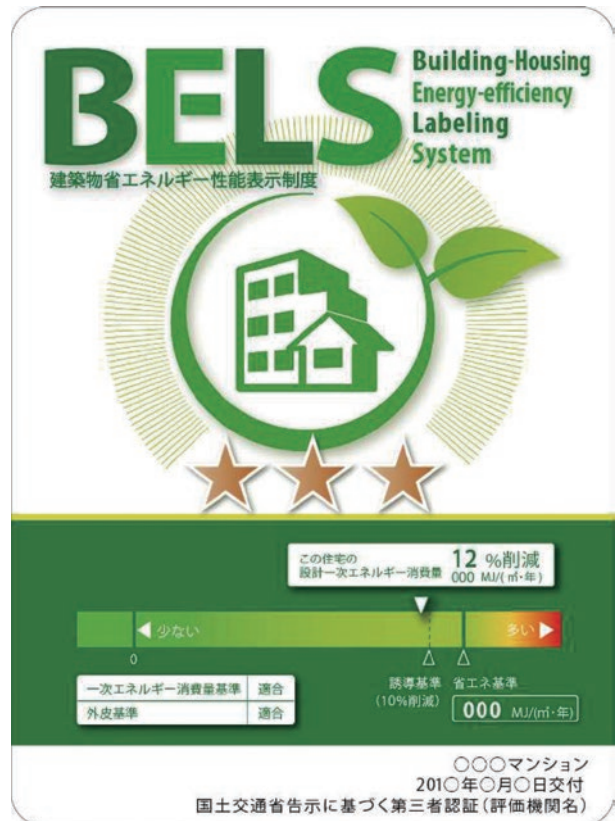
図3-1-5 BELS (Building-Housing Energy-efficiency Labeling System)
