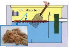
This equipment is installed at the inlet within the grease trap as shown in the left figure. The scumsave net catches the food residues to prevent them from flowing out of the system. The food residues themselves that are caught and
