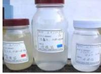
From left, influent, wastewater treated by the device, and effluent from the grease trap
