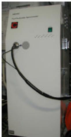
図8 Differential Mobility Analyzer (DMS500)
