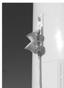
DTBird® Dissuasion Module installed in Greece. View of 2 of the 4 HP Speakers.
