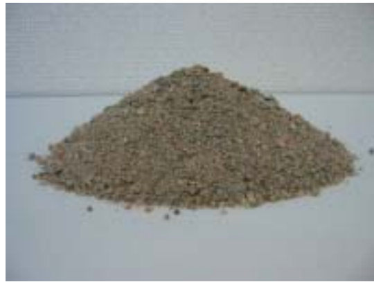
Washed recycled sand
