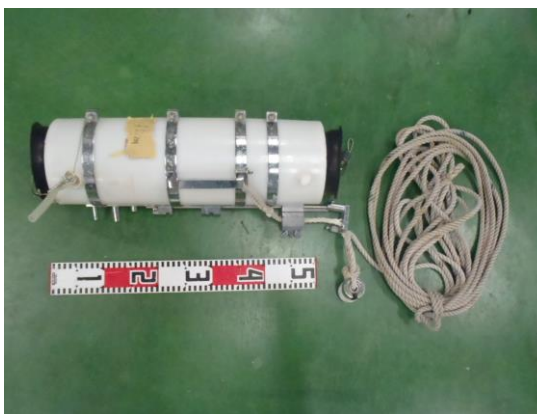
Water Sampler (Example: Van Dorn Sampler)
