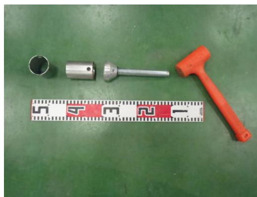
Stainless steel pipe and hammer used for soil collection
