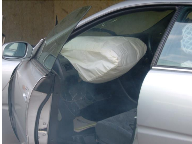
Treatment of air bag in a automobile recycling facility in Osaka, Japan, 2004.
