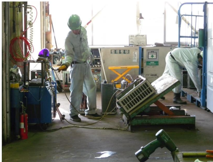
CFC collection from Air Conditioner, Akita, Japan, September 2009.
