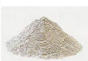
Coal Ash (utilization for cement production)
