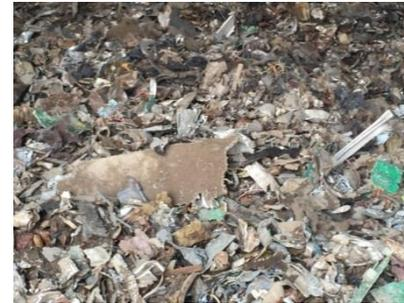
Shredded metals with other materials containing Printed Circuit Boards
