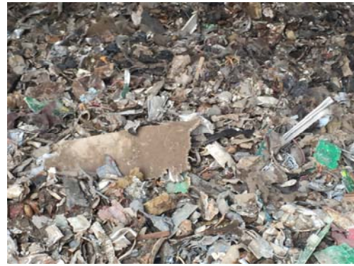
Shredded metals with other materials containing Printed Circuit Boards (PCBs)
