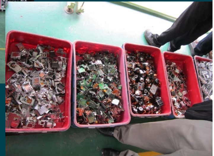
Removed parts for reuse or further recovery
