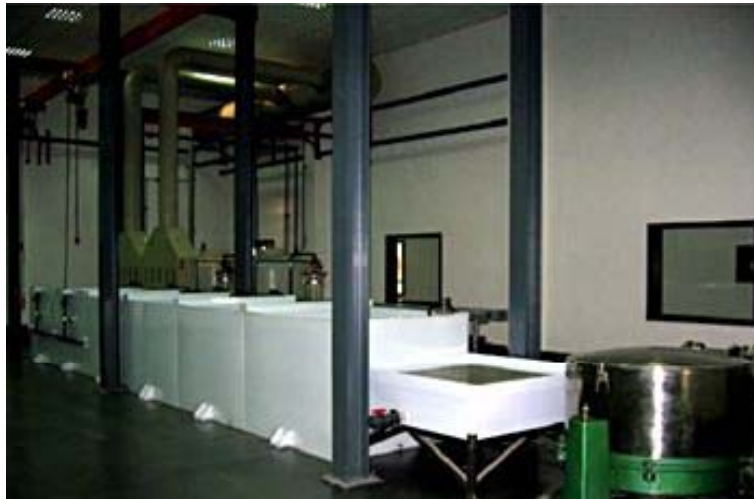
Extraction Process (Stripping) - Stripping of precious metals or metallic coating from base metals
