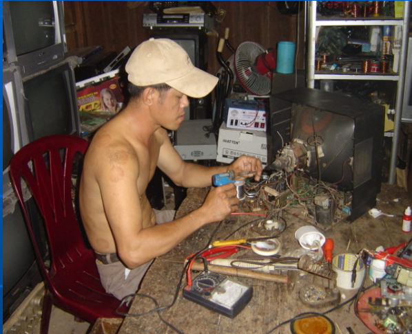
Pic. 21: Unsafe practice for health protection and maintenance during a repairing process, PPM
