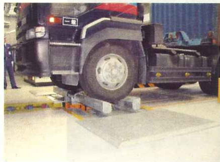
② The container enters into the X-ray machine following the instruction, and the front wheels are lifted up on the traction device.
