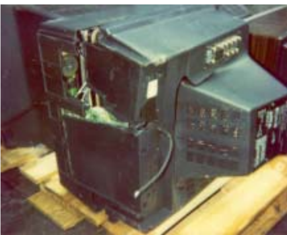
Casing damaged and power cable removed.
