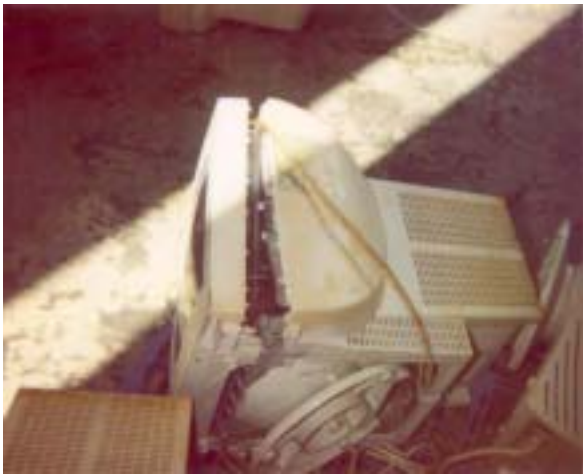
Casing broken and loosened
