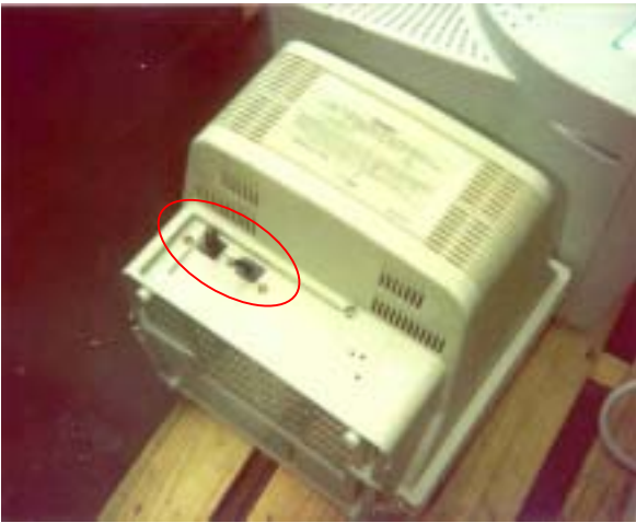
Power and signal cables removed.
