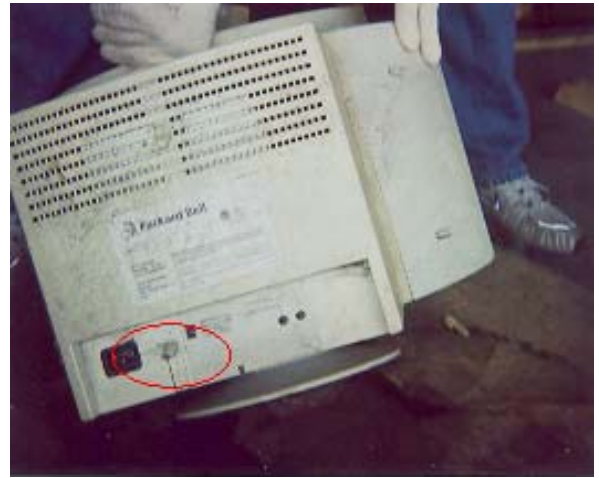
Signal cable removed.
