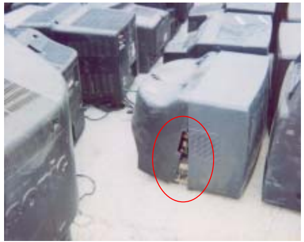
Casing broken and loosened
