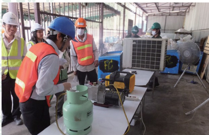
Recovery of fluorocarbons from air conditioners
