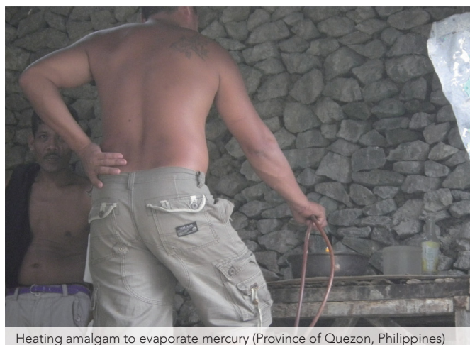
Heating amalgam to evaporate mercury (Province of Quezon, Philippines)
