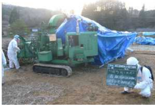
Figure 2-20: Volume Reduction Using a Chipper (Example)
