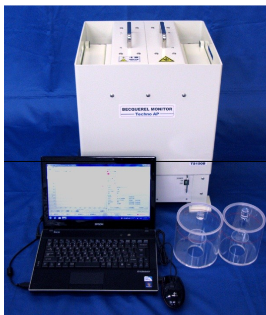
Figure 3-4-3 Example of a LaBr 3 (Ce) scintillation spectrometer
