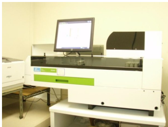
Figure 3-4-2: Example of NaI (TI) scintillation spectrometer
