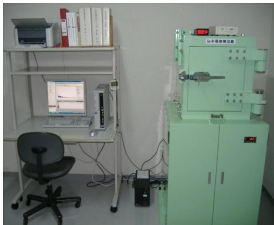
Figure 3-4-1: Example of \Gamma -ray spectrometry using germanium semiconductor detector
