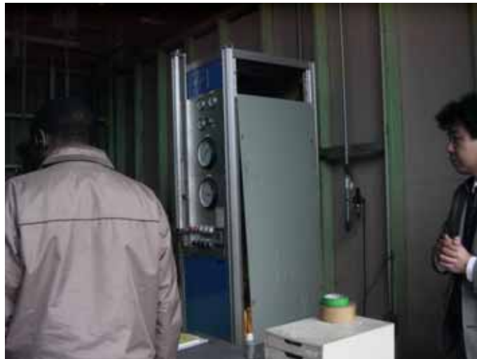
Cylinder strength measurement equipment
