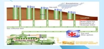
Collection of landfill gas (methane) and its burning in the gas generator for electric power production on one solid waste site of Tashkent city will allow to reduce  $CH_4$  emissions up to 287,2 thousand ton  $C O_2$ /year
